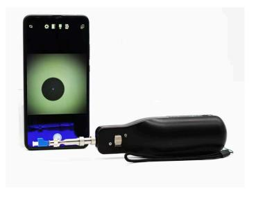
of eight adapters or tips are included to meet all applications of fiber end face inspection analysis. The WIFI-P8 inspection kit includes a wifi inspection probe with rechargeable battery, eight different precision adapter tips, power adapter, user guide, and soft case.
