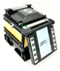
environmental conditions, the WRX12R ribbon fusion splicer will be your trusted tool in the field. Standard features include GPS tracking, automatic arc calibration, fast heating, low loss, 13s splice time, force arc, 100X magnification, reverse monitor, and quick splice mode.
