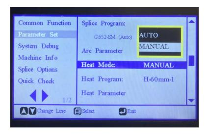
AUTO mode - Place the fiber protective sleeve in the heating box, close the heating box cover and it will heat automatically
