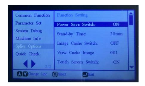
Power Save Switch - machine shuts down automatically after set time
