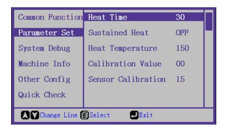
Sustained Heat - Oven will stay on for four minutes in order to heat faster
