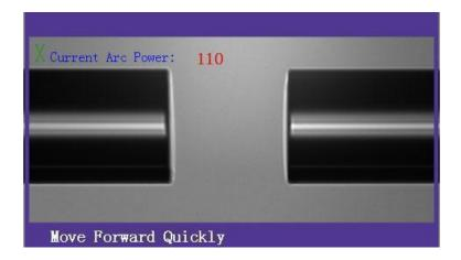
After arc, a numeric value will be displayed on the screen. If the value is within the range of 45-65, it means that the arc power is OK. If the value is less than 45, it means that the arc power is weak, if more than 65, arc power is too strong
