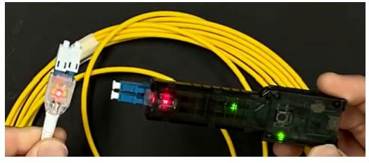
ends to be identified easily without any interruption of service. The separate LED power supply with built-in and changeable battery affixes onto the patch cord keeping it illuminated. Tracker patch cords are available as a 3.0 mm OD duplex LC uniboot style in various lengths in single mode and multimode fiber. The LED Tracker Patch Cords are specified to IEC 61754-20.
